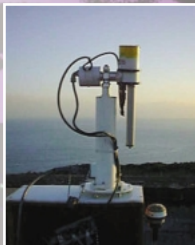
Rame Head Sunphotometer, part of the AERONET global network of sunphotometers measuring direct solar irradiance.
