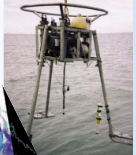
CEFAS seabed lander (Minipod) being deployed from RV Corystes
