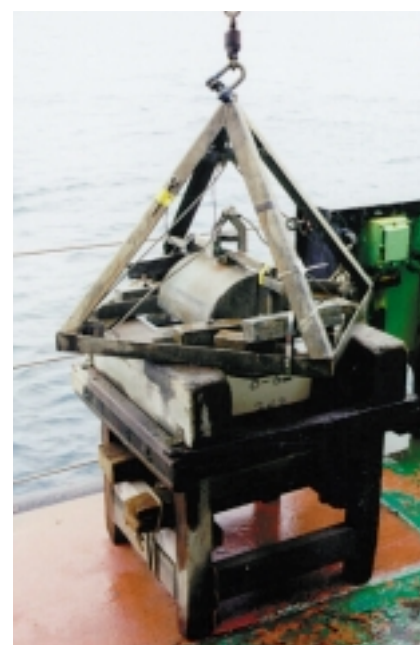
Day grab sampling equipment used to sample the seafloor during the AFEN surveys
