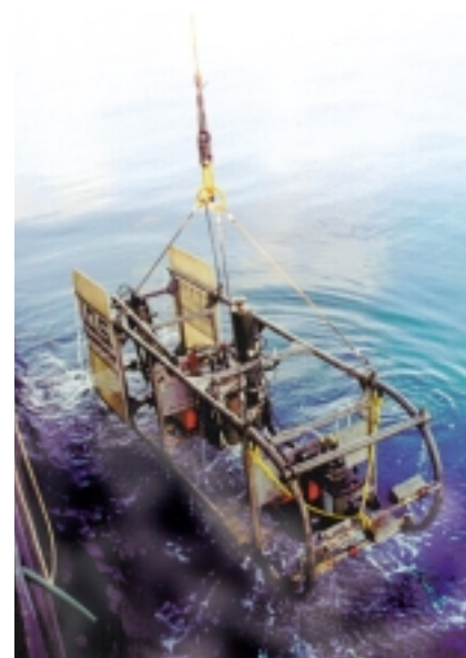
The WASP camera system (Wide Angle Survey Photography) which gives a 'bird's eye' view of the sea bed
